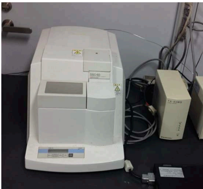
Figure 2.3: Differential scanning calorimetry apparatus used in this present thesis.
