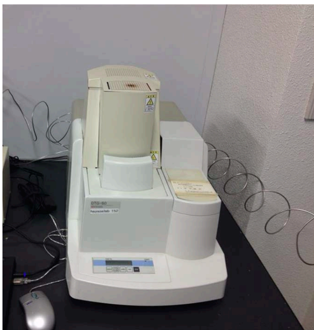
Figure 2.2: Thermogravimetric analysis apparatus used in this present thesis.
