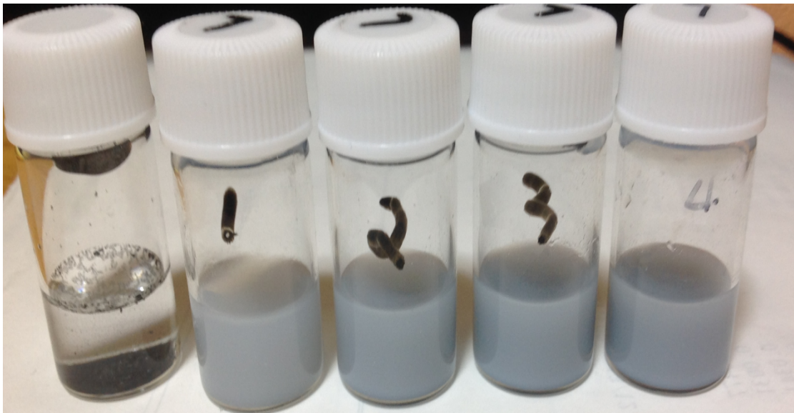
Fig. 35 Pictures of graphene/poly(MMA-co-AEMA)/SiO 2 dispersion in water with different concentration.
