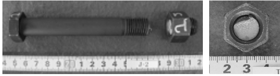
Fig. 4. Specimen ( \alpha=0, \sigma_a=100 \text{ MPa} )
