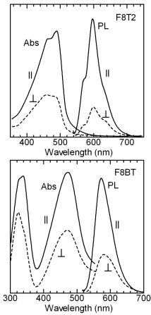
Figure 5: :Polarized absorption and PL spectra of the fluorene based copolymer of (a)F8T2 and (b)F8BT prepared with FTM. Solid and dashed lines represent parallel and perpendicular spectra through a polarizer, respectively.
