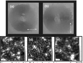
Figure 3: (a), (b): Polarized optical images of a PQT film floated in a petri dish (white arrow as the polarized axis). AFM images of (c):spin-coating film, (d):FTM at 20 °C, and (e):FTM at 60 °C, respectively.
