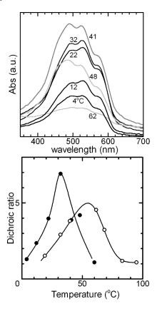
Figure 4: (a):Parallel-polarized absorption spectra of oriented PQT films prepared by FTM at various temperature and (b):temperature dependence of dichroic ratio of the absorption peak at 526 nm.
