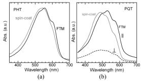
Figure 2: Comparison of absorption spectra of thin films prepared with FTM (black line) and spin-coating (gray line) of (a) PHT and (b) PQT through a polarizer, respectively.
