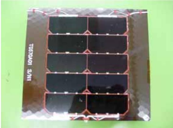
Fig.5. Coupon panel for ESD Testing.
