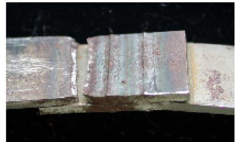
Fig.3 Photo of fracture position (HT980, h=1.6mm)
