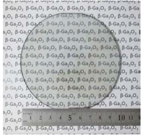
Fig. 23 Photograph of 4"-diameter Ga 2 O 3 wafer.
