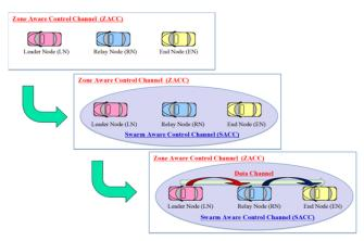
Fig. 3 Procedure of two-hop data communication.
