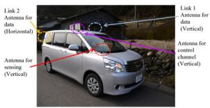
Fig. 5 Antenna setting at RN.
