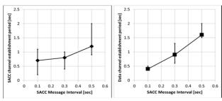
Fig. 13a SACC establishment. Fig. 13b Data channel establishment. SACC messages are periodically transmitted from all nodes in the synchronized manner, our implemented MAC tries to avoid packet collisions. As a result, one SACC interval and processing delay (approximately 100 ms) for frequency change (from ZACC to SACC) are, at least, necessary for the SACC establishment.
