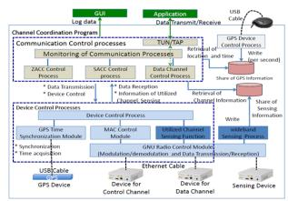
Fig. 6 Architecture for sync. between multiple processes.
