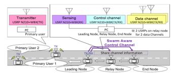
Fig. 4 Hardware components and experimental outline. assigned to a USRP, the management PC can control multiple USRPs simultaneously by specifying an IP address to an individual USRP. From these distinctive points, our implemented system can execute "application communication over data channel", "message exchange over control channel", and "spectrum sensing" in parallel.
