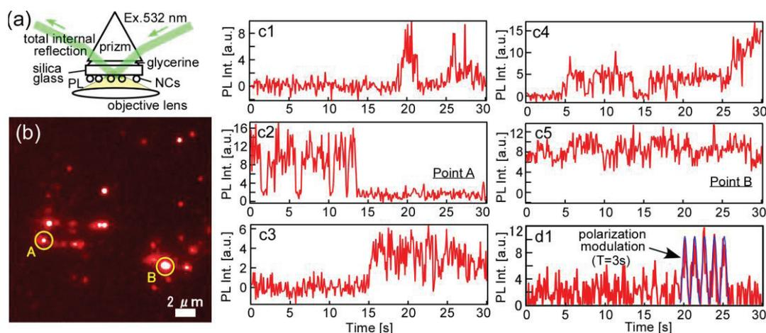
Fig. 4. (a) TIRF excitation configuration of the PL imaging measurement [12]. (b) PL image of the CuInS<sub>2</sub>/ZnS NCs (enlargement of a CCD image of 512×512 pixels). Figs. c1-c5 show the examples of PL time trajectories of each bright spot observed in the CCD image. Fig. d1 shows a typical PL time trajectories under linear-polarization modulation of the PL with rotation speed of 1/3 Hz.
