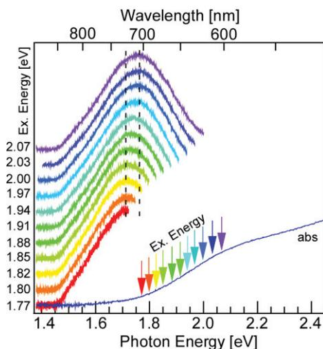
Fig. 2. Excitation-energy dependence of PL spectra of the CuInS<sub>2</sub> NCs with reaction time of 30 min.
