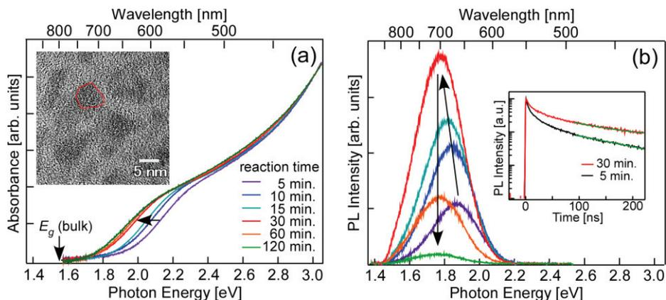
Fig. 1. Reaction time dependence of (a) absorption and (b) PL spectra of CuInS<sub>2</sub> NCs, respectively. The inset of Fig. 1(a) shows a TEM image of the NCs with reaction time of 30 min. Black and red lines in the inset of Fig. 1(b) show PL decay profiles of the NCs with reaction time of 5 and 30 min, respectively.
