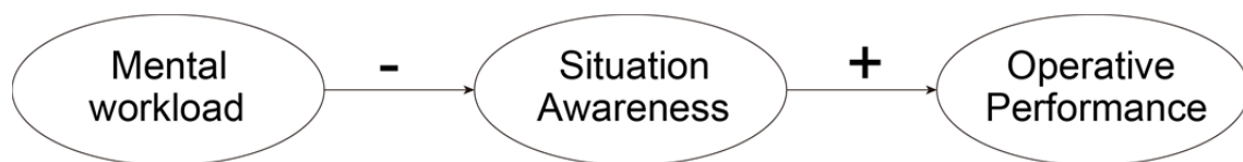
Figure 1.1 An example of the typical relationship between mental state and driver's operative performance. The symbols '-' and '+' represent the relationship (negative correlation and positive correlation) between factors in driving tasks.
