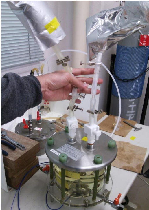
(a) Gas sample was collected in an aluminum bag
