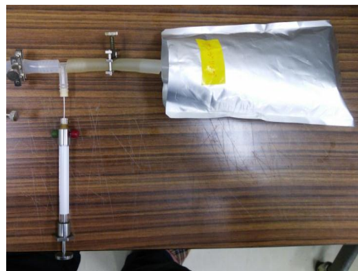
(b) Gas sample was taken using a syringe
