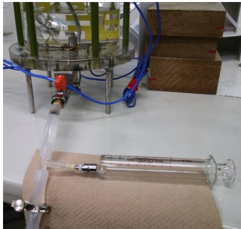
(a) The oil sample is taken from the bottom of the chamber
