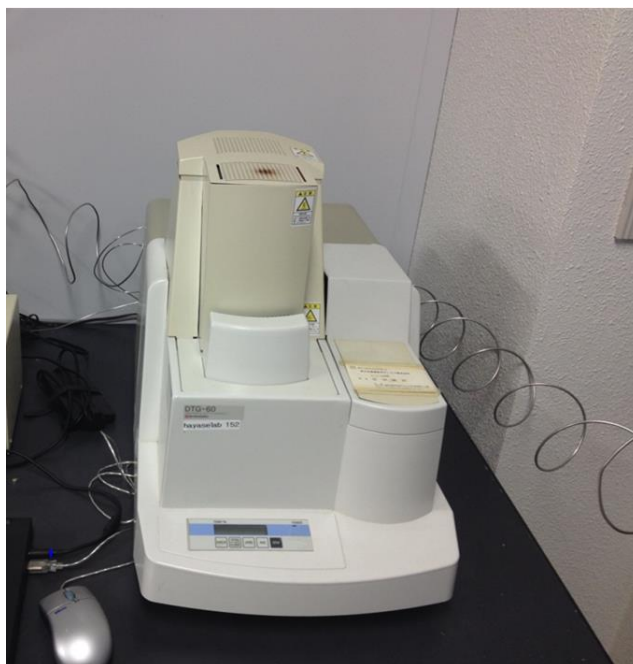
Figure 6. Thermogravimetric analysis apparatus used in this present thesis.
