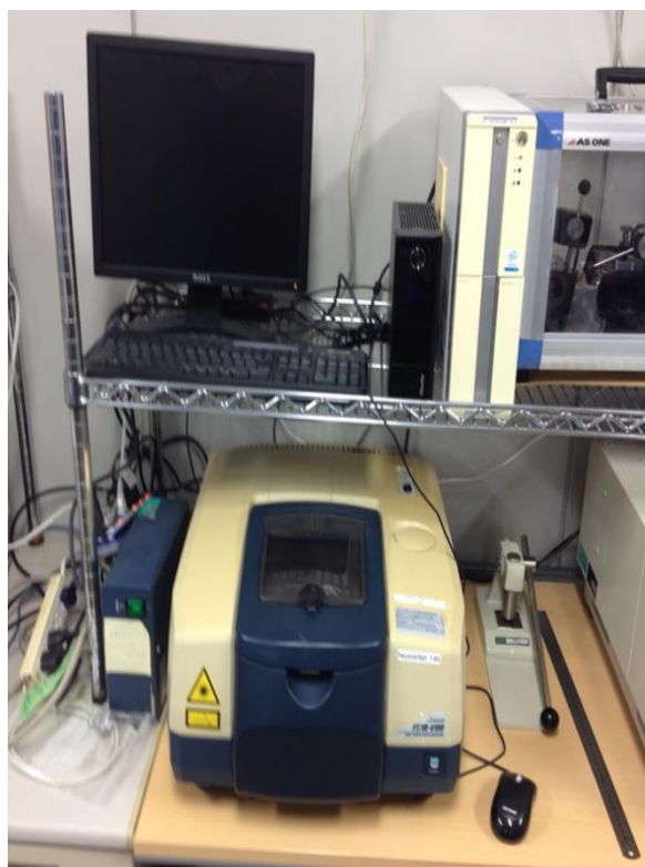
Figure 5. Fourier transform Infrared spectrometer used in this present work.
