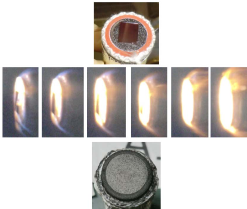
Fig.4-33 Ablator model with solar cell mounted on its front surface
