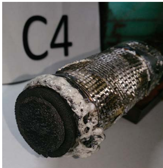
Fig. 4-21 Ablator with density of 500 \text{ kg/m}^3 , after being heated with 13.5 \text{ MW/m}^2 heat flux [4-2]
