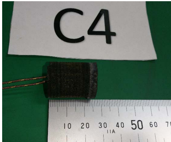
Fig. 4-22 Visualization of the char layer after the test (C4 model) [4-2]
