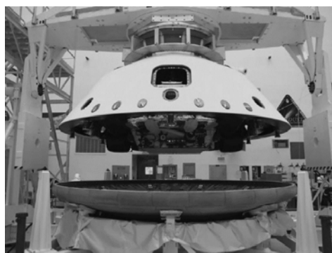
Fig.2-11 PICA tiles for the MSL mission that landed on Mars in Aug. 2012 (Courtesy of JPL/NASA, Reference Figure No. MSL-2011-05-26-143545-img_0959.JPG)
