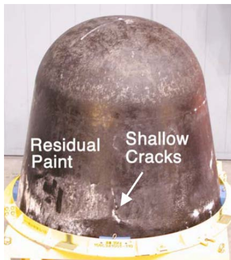
Fig.4-4 Recovered heatshield of USERS. The white spots near are residual paint and dried seawater. [4-5]
