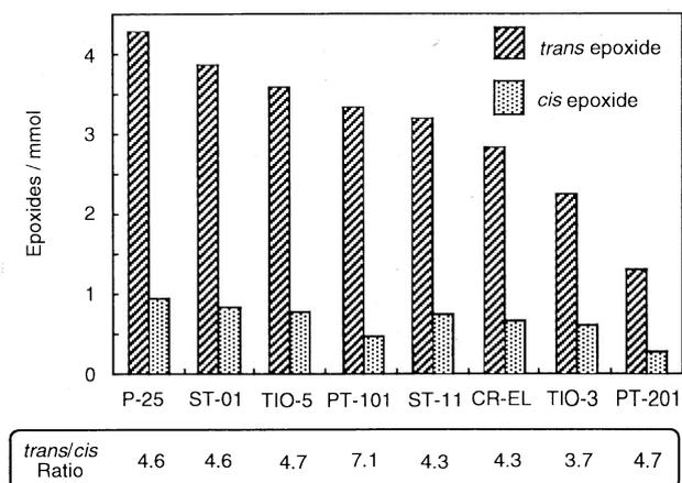
**Figure 2.** Comparison of the photocatalytic activities of different TiO<sub>2</sub> powders for producing *trans*-2,3-epoxyhexane and *cis*-2,3-epoxyhexane from 2-hexene (*trans/cis* = 1.7). The reactions were performed by photoirradiation for 19 h in pure 2-hexene (2.0 g,  $2.4 \times 10^{-2}$  mol) suspended with 20 mg TiO<sub>2</sub> powder under a stream of oxygen.
