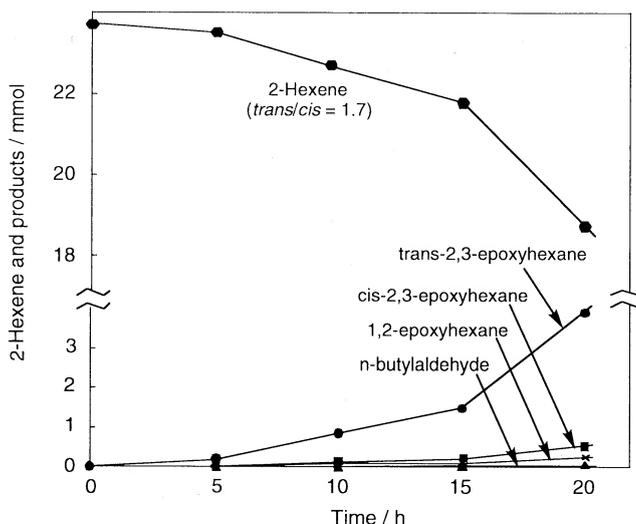
**Figure 1.** Formation of *trans*-2,3-epoxyhexane, *cis*-2,3-epoxyhexane, 1,2-epoxyhexane, and *n*-butylaldehyde as the result of photocatalytic reaction. The reaction was carried out in 2-hexene (*trans/cis* = 1.7, 2.0 g,  $2.4 \times 10^{-2}$  mol) using  $\text{TiO}_2$  powder (Ishihara, PT-101, 20 mg) as the photocatalyst under a stream of oxygen.
