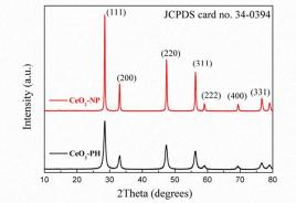
**Fig 1.** XRD patterns of the  $CeO_2$  nanoparticles ( $CeO_2$ -NP), and the  $CeO_2$  porous-hollow spheres ( $CeO_2$ -PH).
