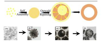
Schem1 formation of the porous-hollow structure; (A), (B), (C), (D) are corresponding to the *Fig S 1*.
