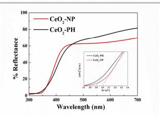
Fig 5. UV-vis diffuse reflectance spectra of CeO<sub>2</sub>-NP and CeO<sub>2</sub>-PH; the inset is the  $(\alpha hv)^2$  versus hv plots curves.
