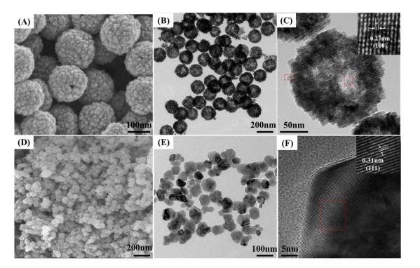
**Fig 2.** SEM images of (A) the CeO<sub>2</sub> hollow spheres, (D) the CeO<sub>2</sub> nanoparticles; TEM images of (B) & (C) the CeO<sub>2</sub> hollow spheres, (E) & (F) the CeO<sub>2</sub> nanoparticles, the inset is the HRTEM images.
