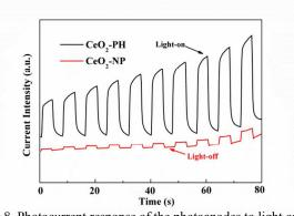
Fig 8. Photocurrent response of the photoanodes to light on-off collected from  $CeO_2$ -NP and  $CeO_2$ -PH electrodes in the solution of 1.0 M Na<sub>2</sub>SO<sub>4</sub> under light illumination.
