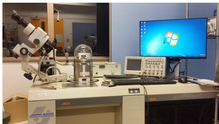
Figure 2.11 Photograph of the JEOL-SPM used for AFM measurement
