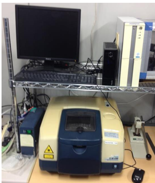
Figure 6. Fourier transform Infrared spectrometer used in this present work
