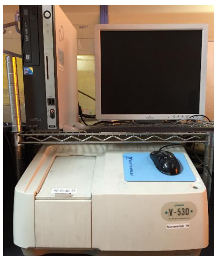
Figure 2. UV-Visible Spectrometer used in the present work
