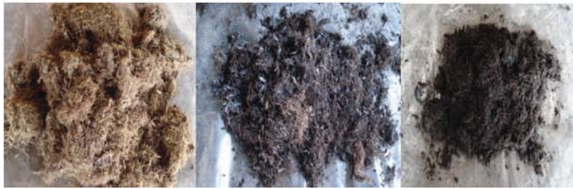
Fig 1: Physical changes during composting; (a) raw OPMF, (b) compost (day 20), and final compost (day 50)
