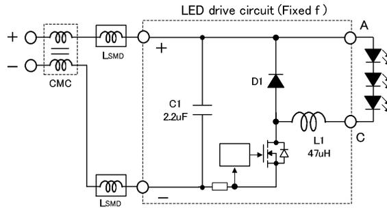
(a) LED Circuit Type 1 Configuration of the N-side Constant Current Control.
