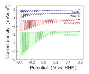
**Figure S2.** Current-potential curves for Pt/CZTS, Pt/CdS/CZTS and Pt/In<sub>2</sub>S<sub>3</sub>/CZTS in 0.1 M NaHCO<sub>3</sub> solution under chopped visible light irradiation ( $420 < \lambda < 800 \text{ nm}$ ,  $100 \text{ mW/cm}^2$ ).
