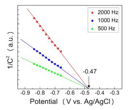
**Figure S3.** Mott–Schottky plots at 500 Hz, 1000 Hz and 2000 Hz measured under dark conditions by using the CZTS electrode in  $Na_2SO_4$  + NaOH solution (pH 9.5).
