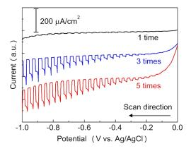
**Figure S1.** Dependence of the photocurrent response of the CZTS electrode on the number of times of spin-coating. The electrolyte was CO<sub>2</sub>-purged 0.1 M NaHCO<sub>3</sub> solution, and light source was Xe lamp attached with cut-off filters ( $420 < \lambda < 800$  nm,  $100 \text{ mW/cm}^2$ ). More than 5 times spin-coating, a crack was appeared in bare CZTS electrode. Thereby, we concluded that 5 times spin-coating is the best for maximum efficiency of the photoelectrode.
