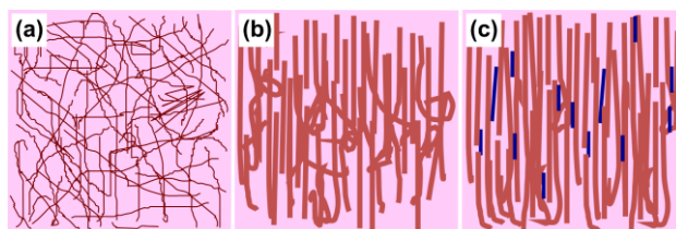
Figure 3. Schematic representation of the thin film microstructures of NR-P3HT coated by (a) as-spun NR-P3HT, (b) FTM coated NR-P3HT and (c) FTM coated NR-P3HT blended with small amount PBTTT (blue stripes).
