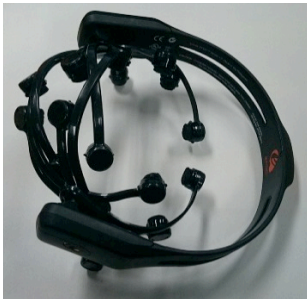
Fig. 1. Emotiv EPOC (wireless portable EEG headset)
