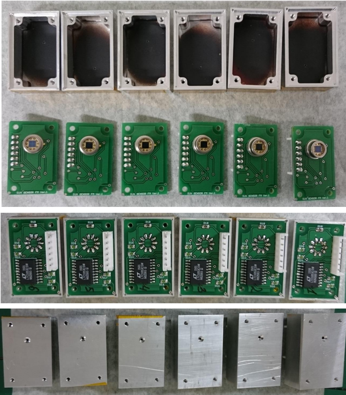
Fig. 2-22. Flight models of sun sensors in assembled and disassembled states.
