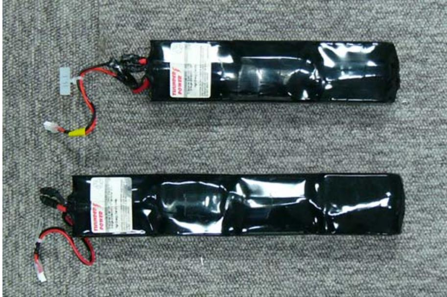
Fig.2-26 Li-polymer Battery(Downside:14.8[V] Upside :11.1[V])
