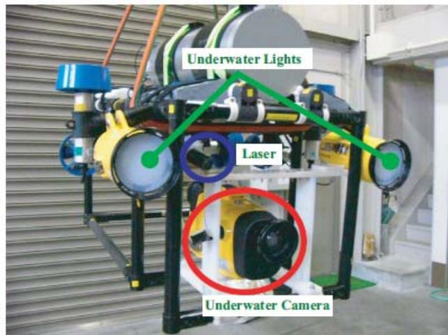
Fig.4-31 Measurement system mounted on AquaBox I
