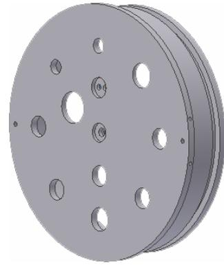
Fig.2-19 Lid of pressure hull (connector side)
