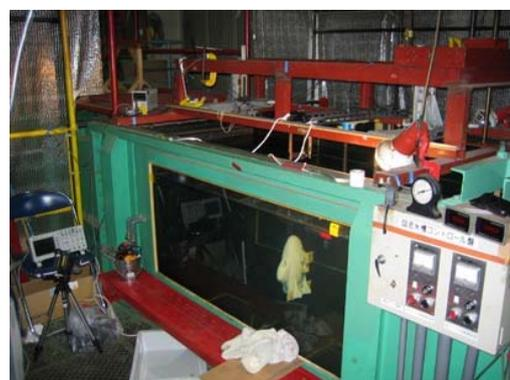
Fig.2-35 Water tunnel (Left-Overall, Right-Observation window)
