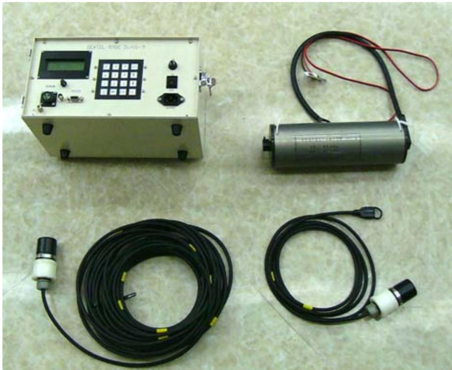
Fig.2-23 Appearance of SEATEL (Left-Land station ,Right-Underwater station)
