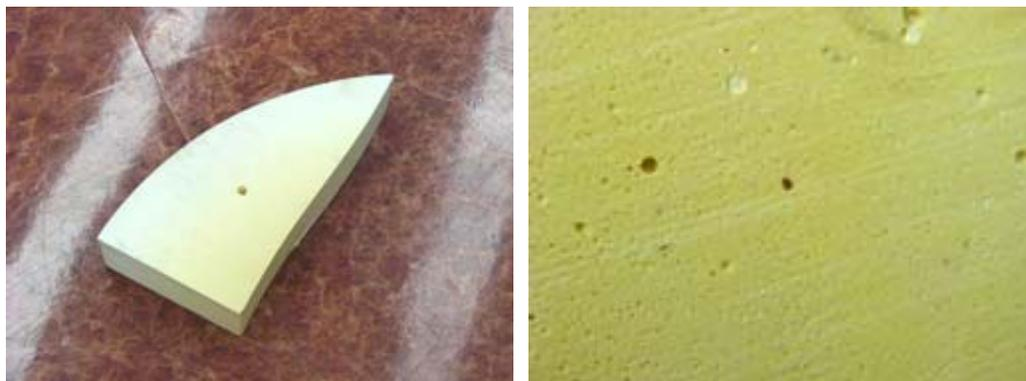
Fig.2-32 Floating buoyant material (Left-Appearance, Right-Surface)
