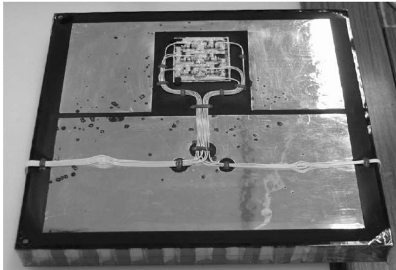
Figure 33: Coupon used for the extreme test. Photograph taken before the test. Damages on Ag-TF film are due to previous tests.
