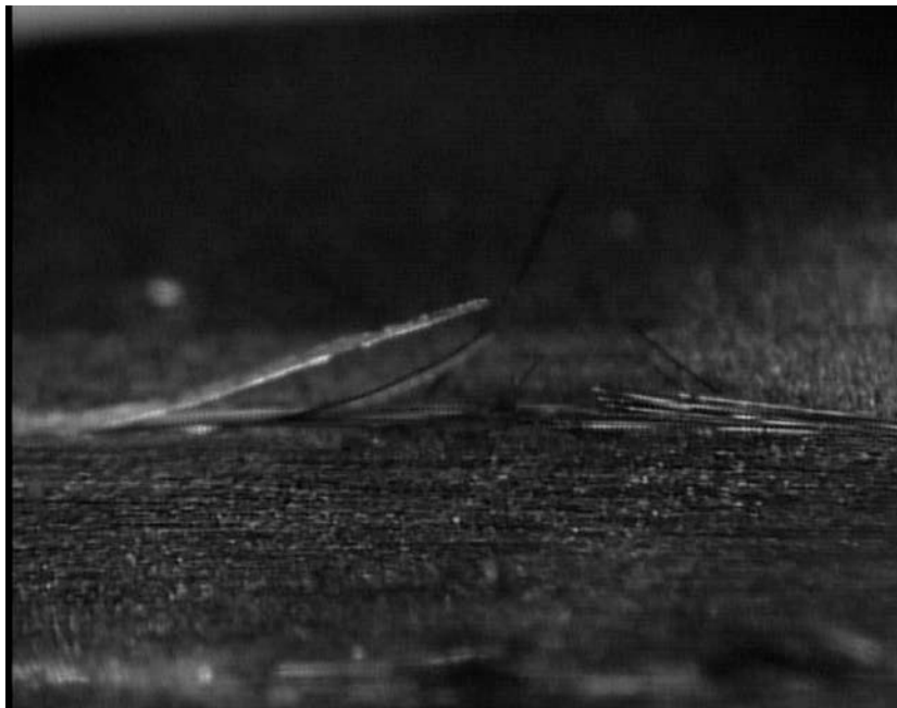
Figure 27: Photograph of protruded carbon fibers from CFRP surface due to primary arcs in plasma environment. The size of photograph is 1.53mm x 1.14mm.
