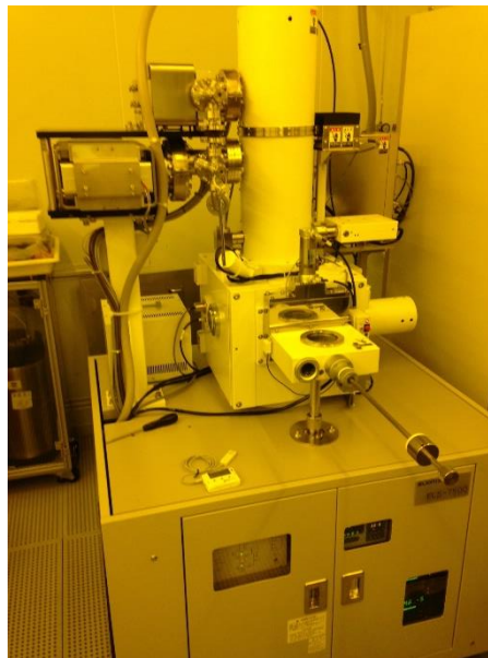
Figure 2. 7 Photograph of EBL machine
