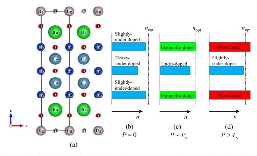
FIG. 9. Possible overview of carrier doping of each CuO<sub>2</sub> plane in the Hg<sub>0.83</sub>(Re<sub>0.18</sub>)-1223 system under hydrostatic-pressure contraction. (a) Structure of the unit cell and carrier doping level at (b) P = 0, (c)  $P \sim P_c$ , and (d)  $P > P_c$ .
