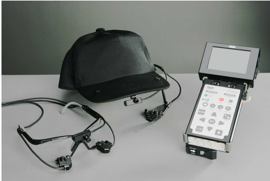
Figure 1.10: Gaze estimation device from Nac image technology. (Left: EMR-9 CAP; Middle: EMR-9 Glasses; Right; EMR-9 Controller) [10]
