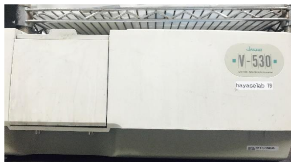
Figure 4. UV-Vis spectrometer used for measuring the electronic spectra of the compounds discussed in the thesis.
