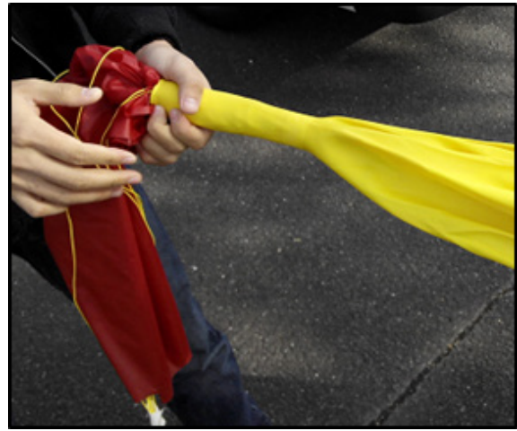
Figure 17. Insertion of Parachute into Balloon
