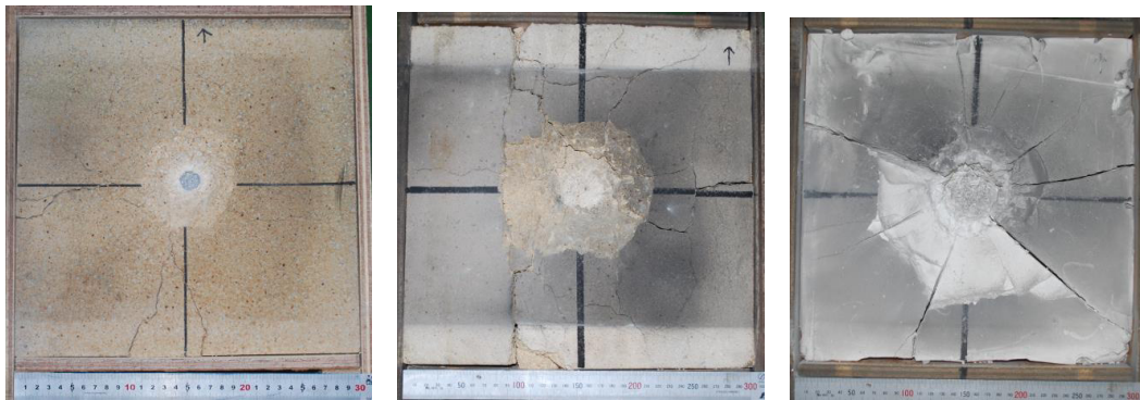
Fig.7. Images of targets after impact: left shows target of LTS14-052 (L300mm×W300mm×T140mm, 28.26kg, crater diameter is 100mm, crater depth is 13.91mm, ejecta* is 190.0g); center shows target of LTS14-053 (L300mm×W300mm×T200mm, 38.84kg, crater diameter is 145mm, crater depth is 29.48mm, ejecta* is 51.0g); right shows target of LTS14-054 (L300mm×W300mm×T180mm, 17.87kg, ejecta* is 168.8g); * only collected.
