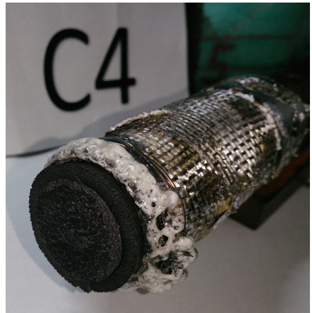
Fig. 6. Ablator with density of 0.5 g/cc, after being heated with 13.5 MW/m 2 heat flux.
