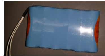
Fig. 6. A pack of six series connected Eneloop ® NiMH cells.
