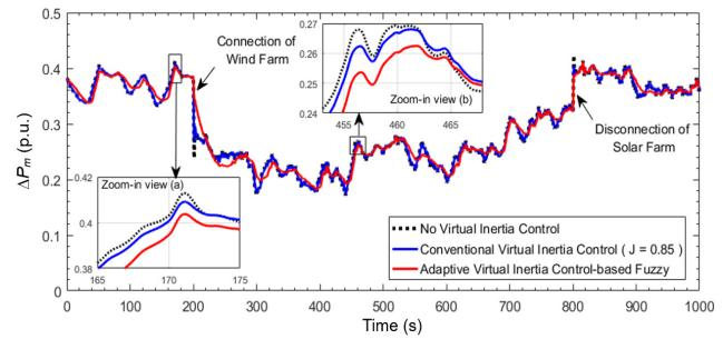
**FIGURE 10.** Thermal power response for scenario 1.
