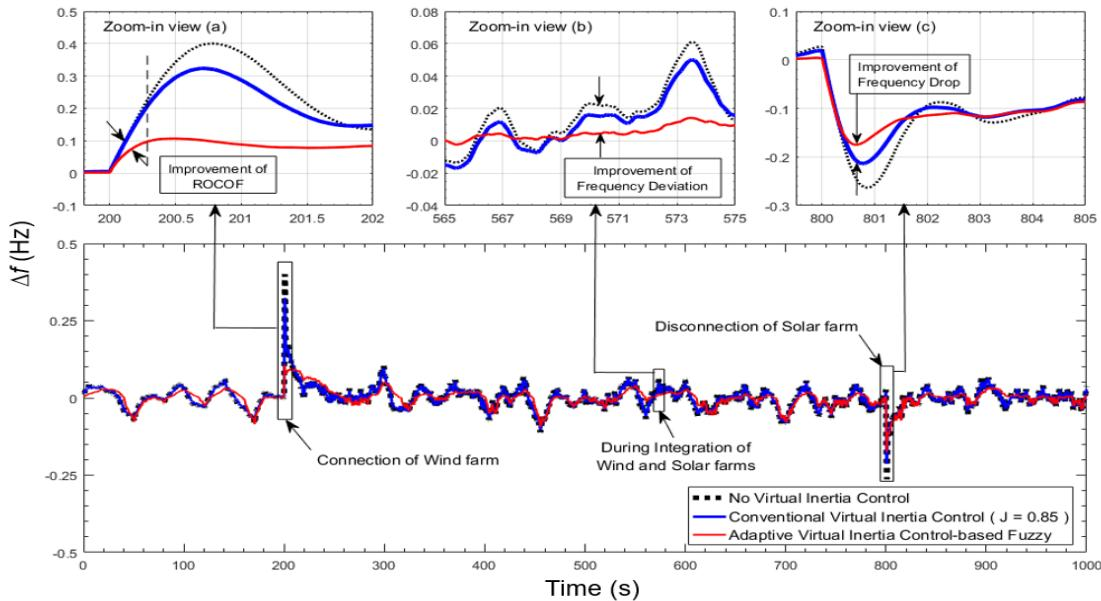
**FIGURE 8.** Microgrid frequency response during low RESSs penetration corresponding to high system inertia (scenario 1).
