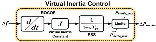
**FIGURE 3.** The dynamic model of virtual inertia control.
