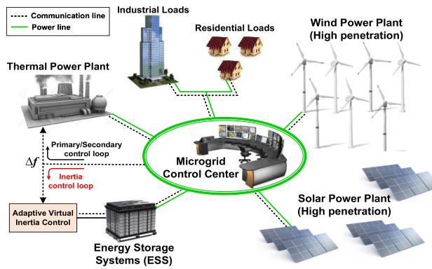
**FIGURE 1.** The simplified model of the studied microgrid.
