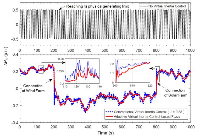
**FIGURE 13.** Thermal power response for scenario 2.
