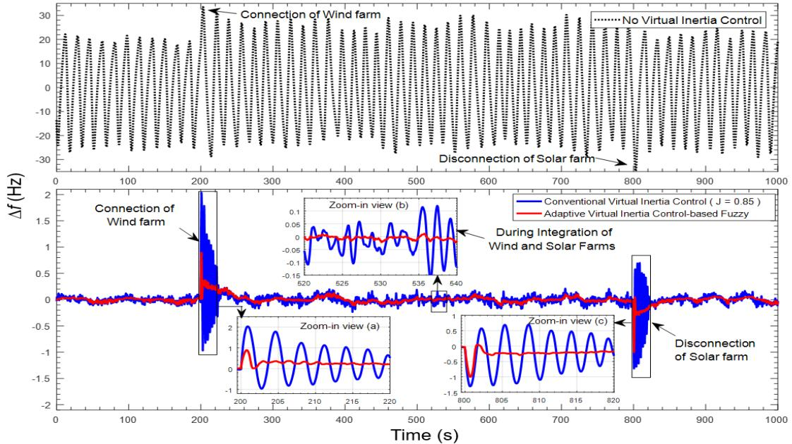
**FIGURE 15.** Microgrid frequency response during the mismatch primary/secondary control and microgrid parameters (Scenario 3).
