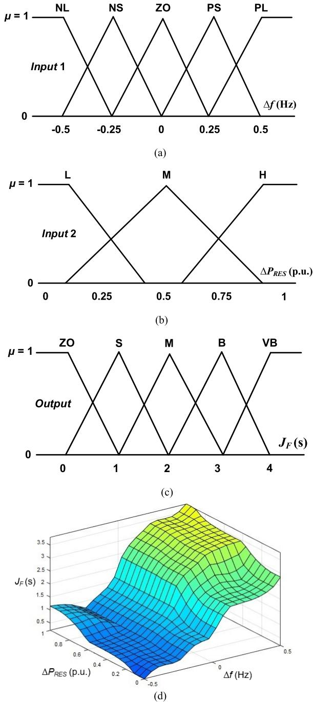
**FIGURE 6.** Symmetric fuzzy membership functions: (a) System frequency deviations. (b) RESs power changes/penetration. (c) Virtual inertia constant. (d) Effect of RESs penetration and system frequency deviations on the output of the fuzzy system.
