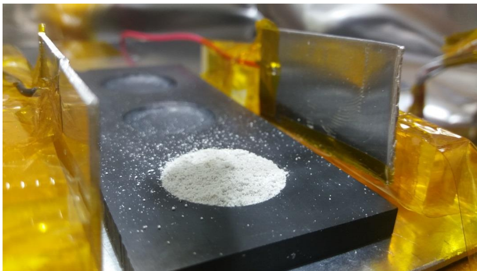
Figure 4.22 : Test environment schematic (top) and dust sample between the parallel aluminum plates (bottom).
