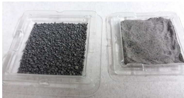
Figure 1.7 : Japanese lunar simulant separated by sifting process in the laboratory.
