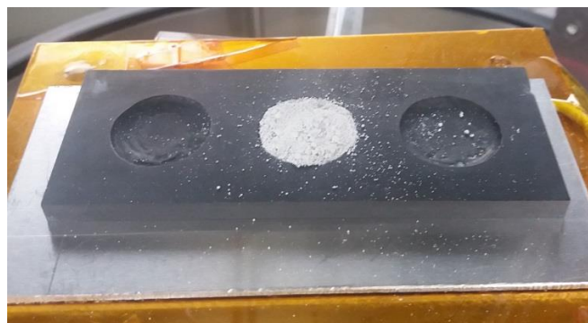
Figure 4.12 : Scattered silica dust grains on the graphite plate after the exposure to the electron beam current.
