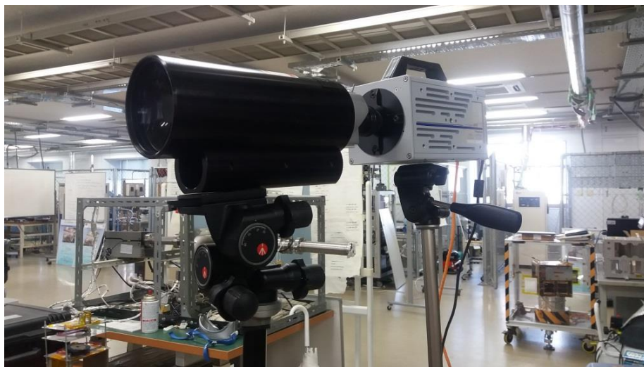
Figure 4.2 : The microscopic telescope and the high-speed camera.
