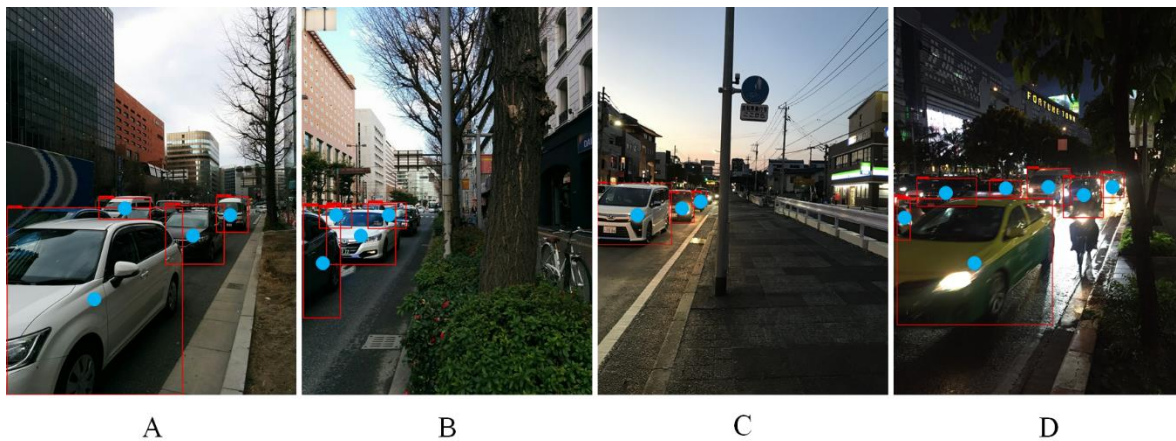
Figure 5.6 Outcomes of car detection using the YOLOv2 technique (these images are related to the graphs of Figure 5.7).
