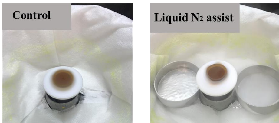
Figure 5-2 One-step anti-solvent method for preparing perovskite films. (a) Conventional process and (b) liquid nitrogen assist process, the ambient temperature is about 23 °C and the temperature during spin-coating was about 4 °C.
