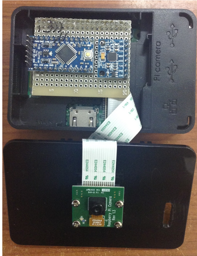
FIGURE 3.15: Assembled hardware of prototype of Vision-based attitude sensor.
