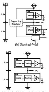
(c) Stacked-Vdd with I/O Coding Fig.1 Circuit Configuration
