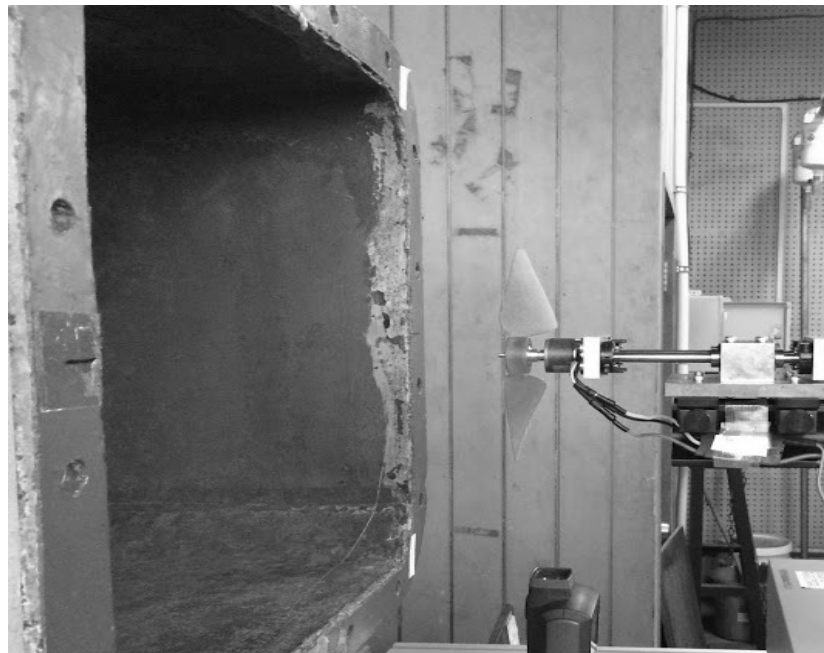
Figure 3-7: Propeller on Wind tunnel test stand ( Thrust test configuration)
