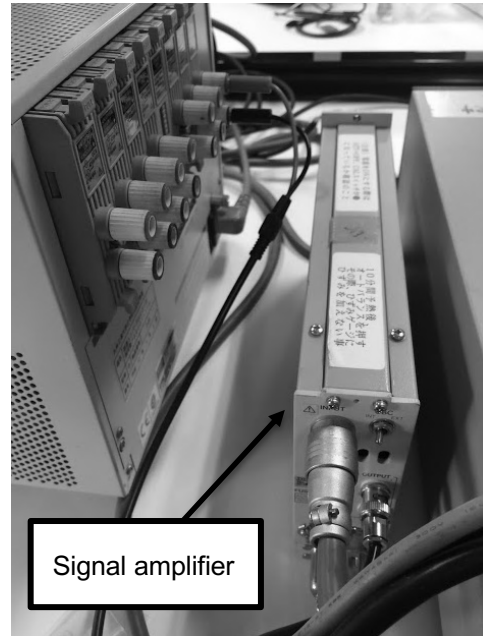
Figure 2-11: Oscilloscope (a) and Signal Amplifier (b) used to collect data from strain gauge in the measurement of thrust
