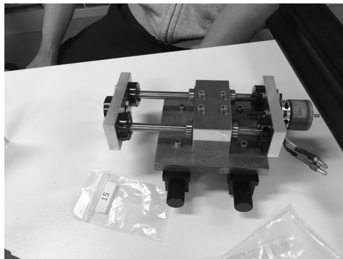
Figure 2-10: Frictionless 1 axis slide bushing for thrust measurement
