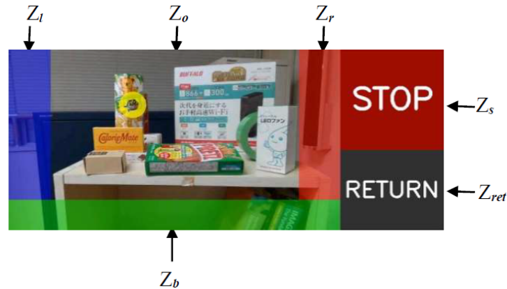
FIGURE 4. Developed graphic user interface for human-robot communication: The screen of a PC is separated into 6 colored zones.
