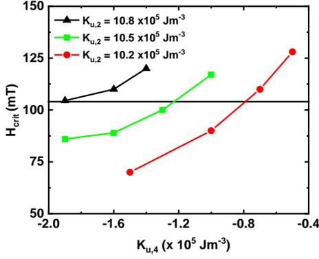
Fig 4. Switching fields  $H_{s0}$  as a function of 4<sup>th</sup> order perpendicular anisotropy energy  $K_{u,4}$  for different values of second order perpendicular anisotropy fields  $K_{u,2}$ .
