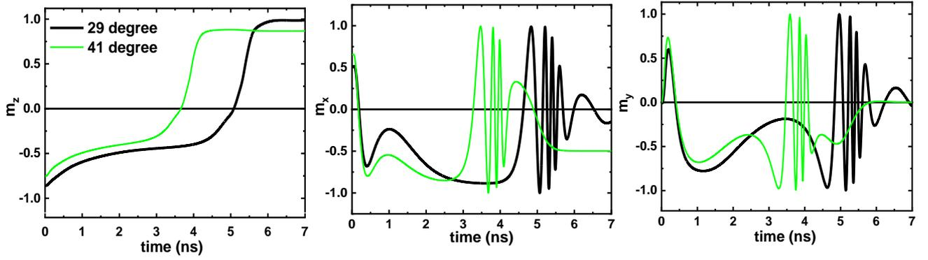
Fig 6. Time evolution of the (a) z- component  $m_z$ , (b) x-component  $m_x$ , and (c) y-component  $m_y$ , of magnetization vector when a z-axial field pulse  $H_{s0} = 104$  mT is applied on a sample with  $\theta = 29$  degree (S-3) and  $\theta = 41$  degree (S-5). Rise and fall times of the pulse are 0.1 ns and pulse duration is 10 ns.
