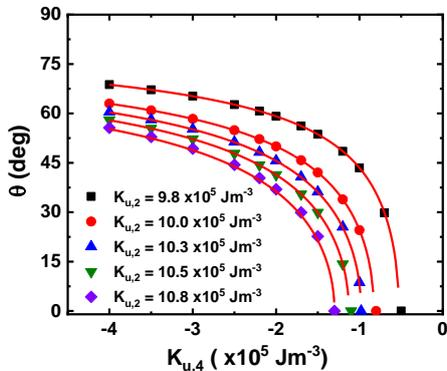
Fig. 2. Evolution of  $\theta$  as a function of the second  $K_{u,2}$  and fourth  $K_{u,4}$  order perpendicular magnetic anisotropy energy (symbols) for a thin film with a fixed saturation magnetization  $\mu_0 M_s = 1.5$  T. Lines are fits to (2) in the main text.
