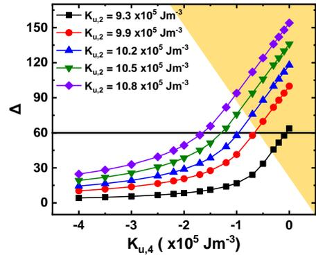
Fig. 3. Evolution of thermal stability  $\Delta$  as a function of the second  $K_{u,2}$  and fourth  $K_{u,4}$  order perpendicular magnetic anisotropy energy for a thin film with a fixed saturation magnetization  $\mu_0 M_s = 1.5$  T.
