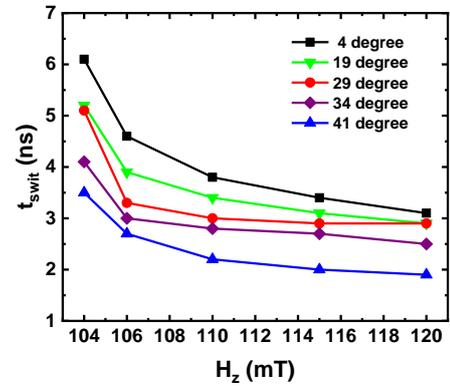
Fig. 5. Switching time  $t_{\text{swit}}$  as a function of the amplitude of the field pulse  $H_z$  which shows a longer switching time for sample with  $\theta = 4$  degree (S-1),  $\theta = 19$  degree (S-2),  $\theta = 29$  degree (S-3),  $\theta = 34$  degree (S-4) and  $\theta = 41$  degree (S-5).
