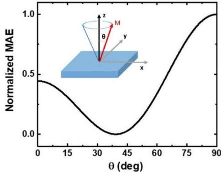
Fig. 1. Schematic to illustrate the magnetic anisotropy energy (MAE) as a function of the angle of the magnetization from the film normal  $\theta$  for a thin film with an easy cone state. Inset shows the coordinates used in the study along with a definition of  $\theta$ .
