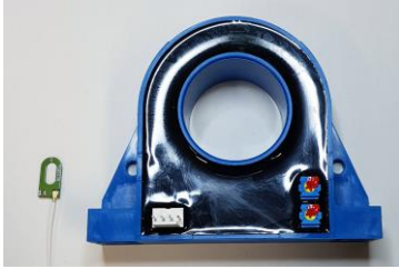
Fig. 2. Miniature (green) PCB coil and conventional current sensor.
