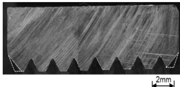
Fig. 3-2 Chamfer usually used for standard nuts larger than M6(JIS).
