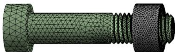
Fig. 3-7 FEM model for M10 bolt
