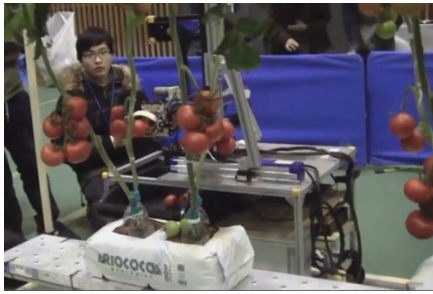
Fig. 5 The winner robot of the 6th competition, Kyutech team. The robot harvested 5 tomatoes in the final stage.
