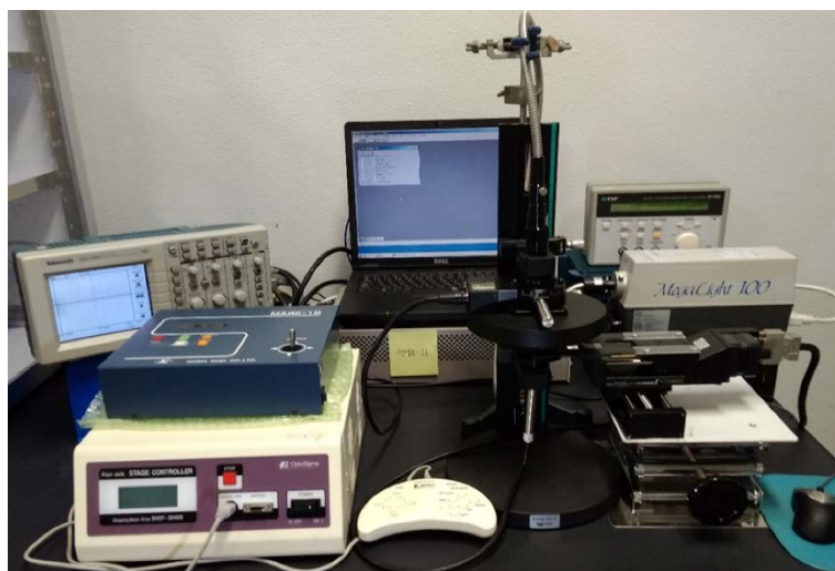
Figure S1. Digital image of the custom-made set up for 2D positional mapping.
