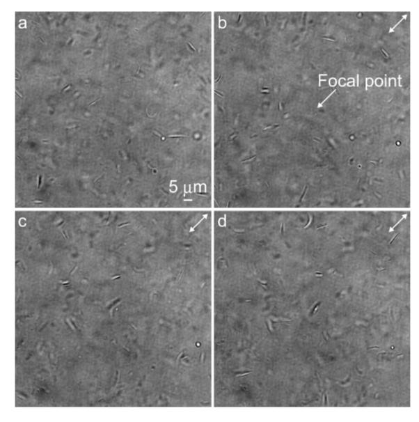
Figure 2. Optical microscopy images of a niobate nanosheet colloid (a) before laser irradiation and after (b) 15 s, (c) 30 s, (d) 34 s of continuous laser irradiation with a linearly polarized laser beam. The very small white point shown in (b) represents the focal spot with a diameter of  $0.4 \mu m$ . The white arrow indicates the polarization direction.
