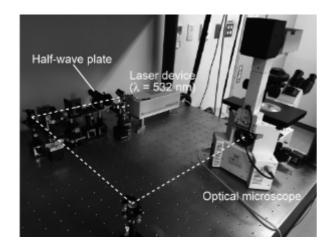
Figure 1. Photograph of the experimental setup. The broken line indicates the beam path
