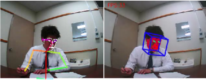
Fig. 2. Estimated information by OpenPose (left) and OpenFace (right)
