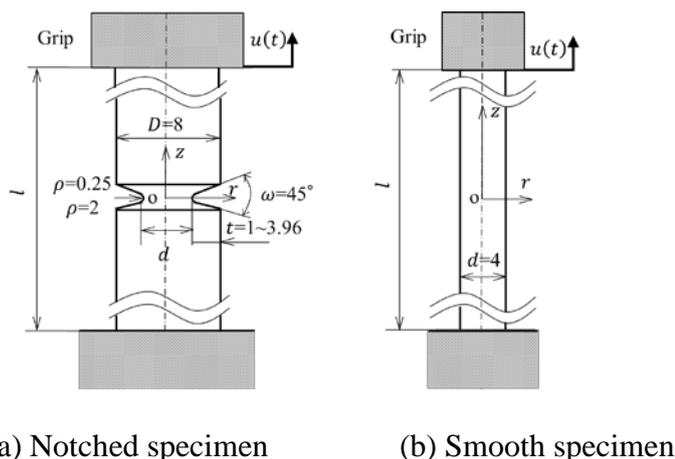
Fig. 1. Geometry of specimens (Dimensions: mm)
