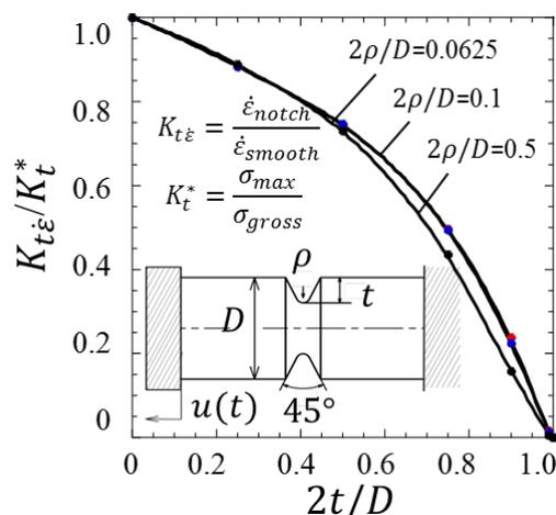
**Fig.5.** Relationship between  $K_{t\dot{\epsilon}}/K_t^*$  and  $2t/D$  when  $l/D=5$  ( $l=40\text{mm}$ ,  $D=8\text{mm}$ )
