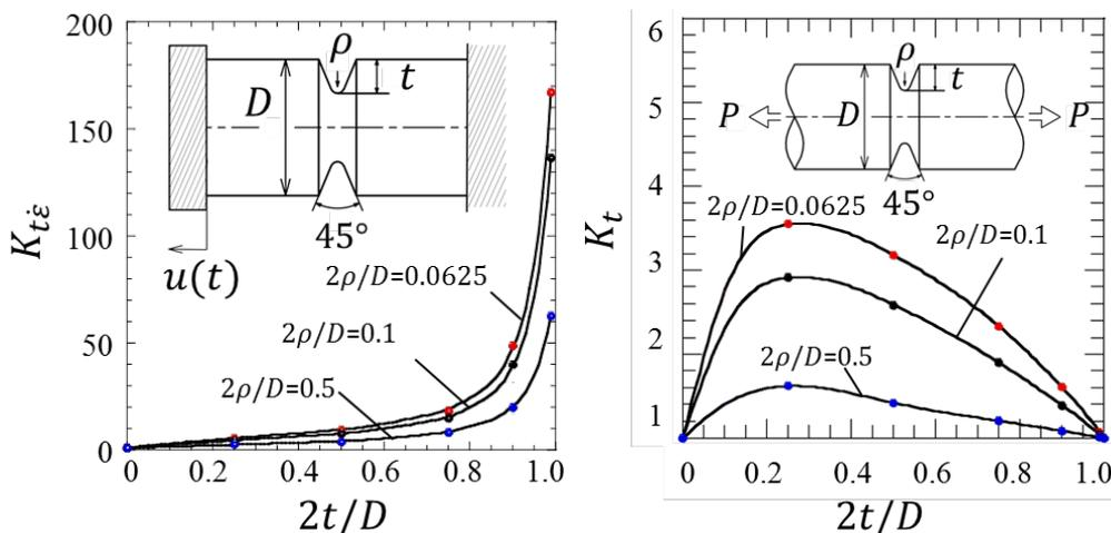
(a) Relationship between  $K_{t\dot{\epsilon}}$  and  $2t/D$  when  $l/D=5$  ( $l=40\text{mm}$ ,  $D=8\text{mm}$ )      (b) Relationship between  $K_t$  and  $2t/D$  when  $l/D=5$  ( $l=40\text{mm}$ ,  $D=8\text{mm}$ )
