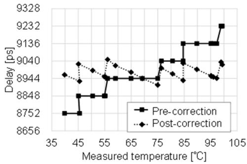
Figure 13. Delay measurement under variable temperature
