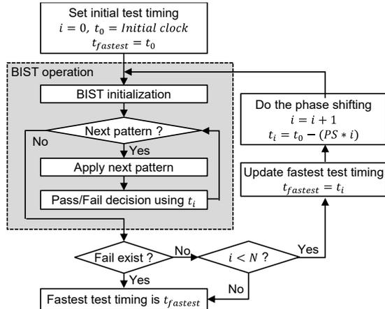
Figure 6. Flow of the delay measurement with variable test timing
