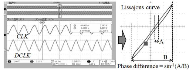
Figure 9. Observation of the phase difference between an original and a controllable clocks using Lissajous waveform.
