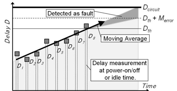
Figure 1. Delay measurement for degradation detection in-field [17]
