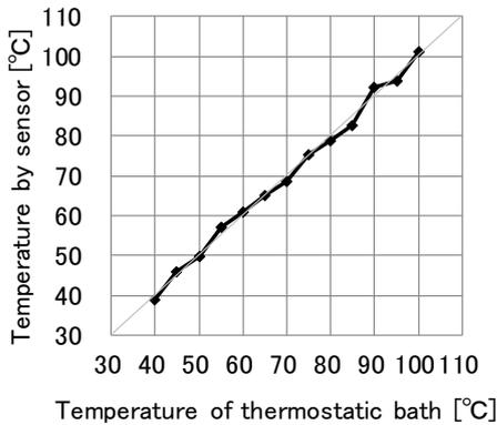
Figure 11. Evaluation of a temperature sensor
