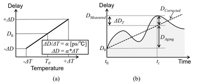
Figure 7. Relation between the measured delay, the temperature, and the delay increasing due to aging in field.
