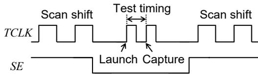
Figure 3. Test timing of Launch-off-Capture
