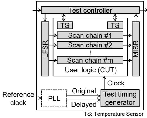
Figure 2. Design structure of delay measurement with LBIST
